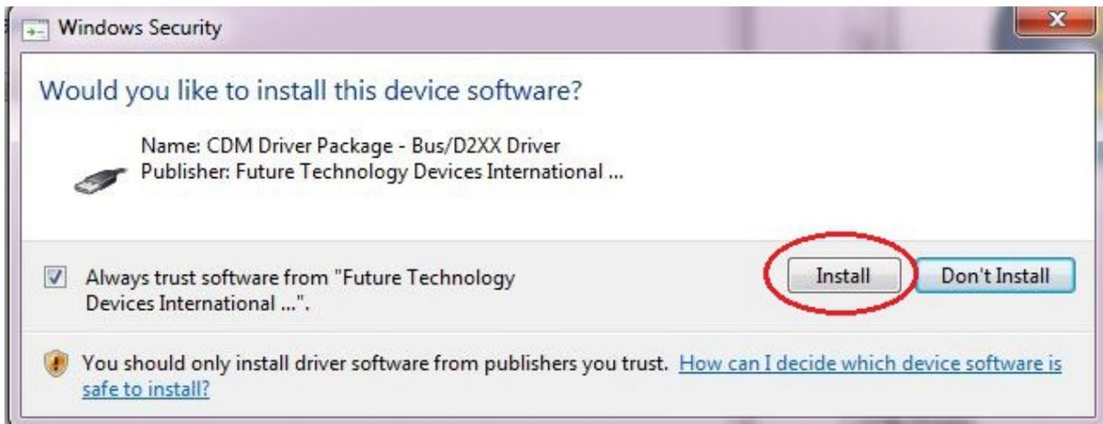
If the installation is successful, the PC recognises the device as an USB Serial (COM) Port.
