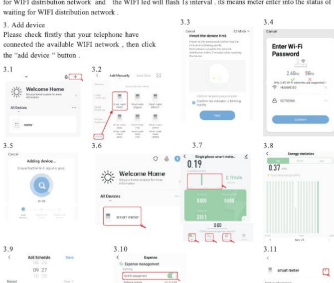
If device connect successfully ,you can realize remote control on/off, timer control and delay time control, and read the energy /current/ voltage/active power and history energy. you also can change the device name and share the device to others. If closed the prepayment function ,the balance energy will reset zero.
